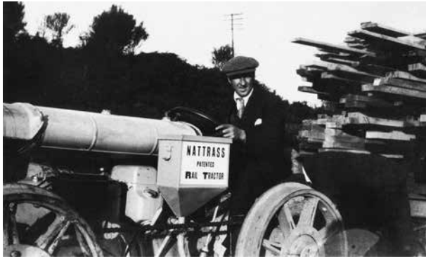
A Nattrass Patent Rail tractor operated on the Taringamutu Totara tramway in 1925 but according to Henry McHattie, it was a failure. This photo shows the machine hauling some sawn timber to the railway station and whilst it moved a considerable amount of timber, the hierarchy at Taringamutu Totara Sawmills were not impressed.
