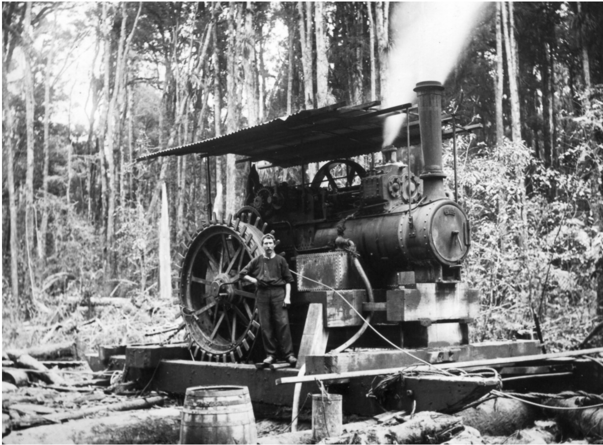
This photo shows a traction engine set up as a hauler. The front wheels have been removed and a sturdy frame built to support the machinery. The main hauling rope is wound onto the large rear wheel. This main rope was pulled out to the logs by horses. This set-up was first used at the Otorohanga workings of E&B and then at the bush workings on Tiroa. For its day it was quite a satisfactory method of hauling in the logs. A W Bathgate photo from the Richard Stratford collection.
