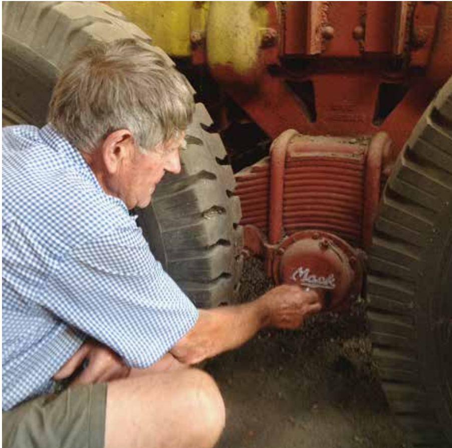
Ross Hopkins carefully chalks the maker's logo to make it stand out for this photograph. He says the back end of the Mack model NO-2 is in good condition despite spending over a decade of its life under water. Ross pointed out that the leaf spring assembly used in the tandem suspension was commonly known as a "camelback" due to its central hump.
