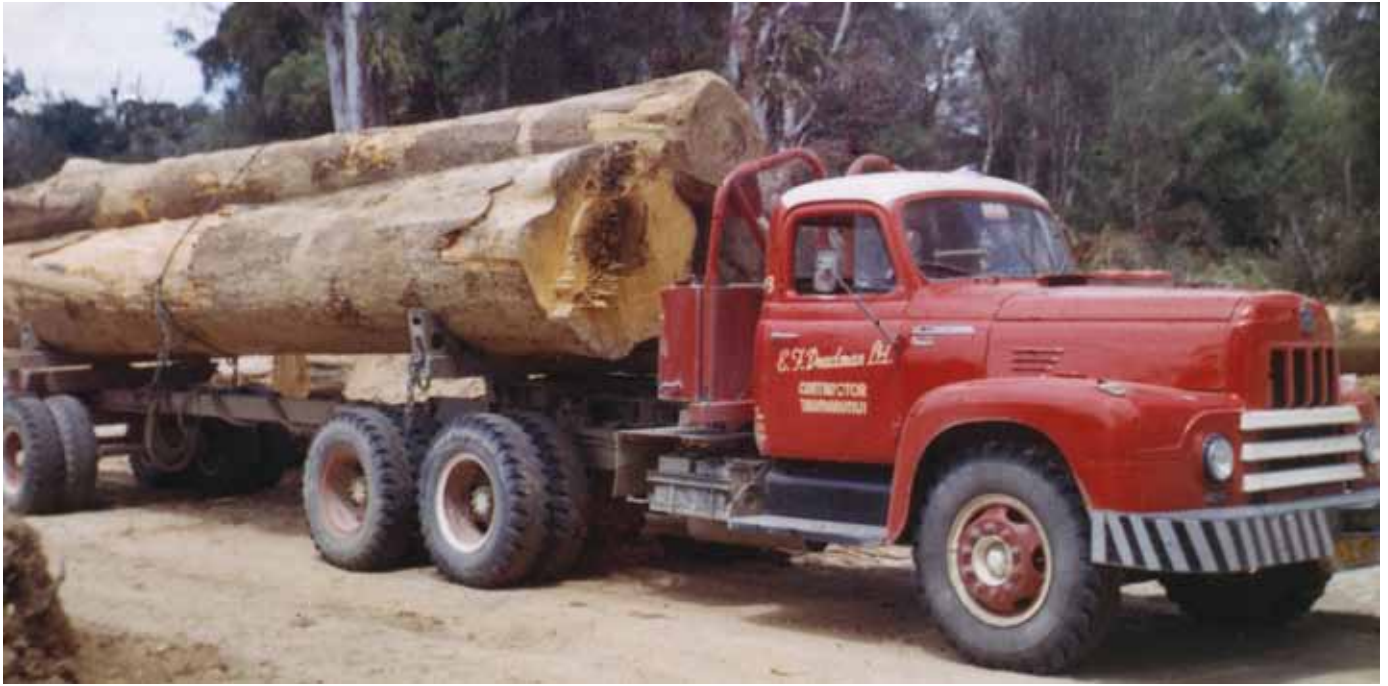
Eric Deadman's R195 International had its bonnet extended by Ross Todd Motors to fit a new 6-71 GM diesel motor with the body modifications being of such high standard that it is almost impossible to detect any changes. Eric was so happy that he had two more trucks fitted out by Ross Todd.
