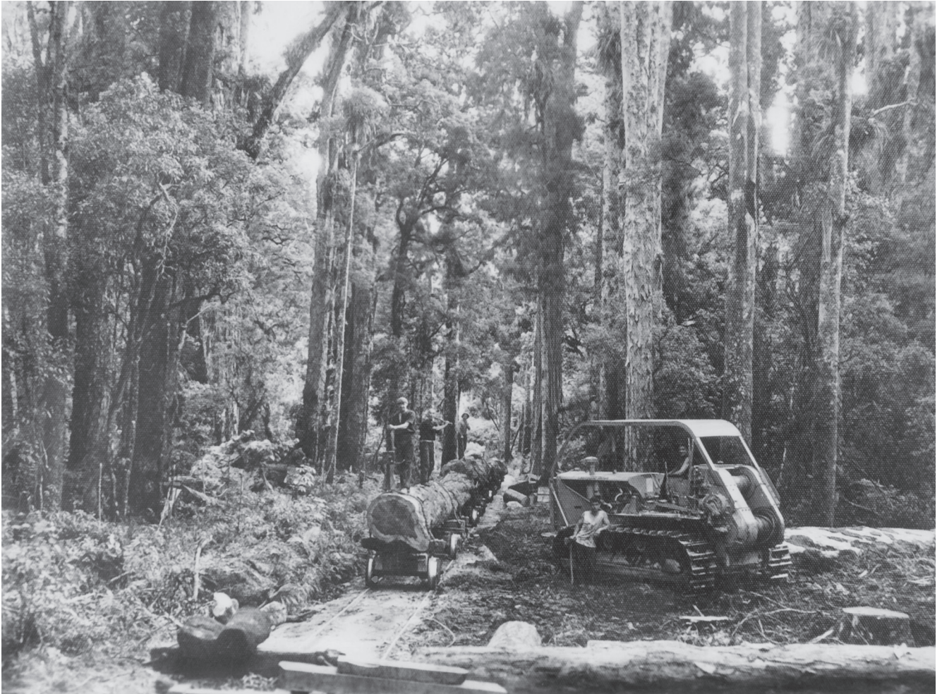
The first big tractor in the area – the Diesel 75 on the loading skids in the bush at Pukemako. The tram bogies have been loaded and the tractor will shortly go out for another drag. The first man on the rear log has a timber jack and this would have been used to load the logs. Later a Caterpillar Twenty tractor arrived to assist with the loading. It is likely that this photo was taken when GG&H were contracting for Ellis & Burnand. By 1936 this tractor was at Ongarue. What fine timber there is in the background.
