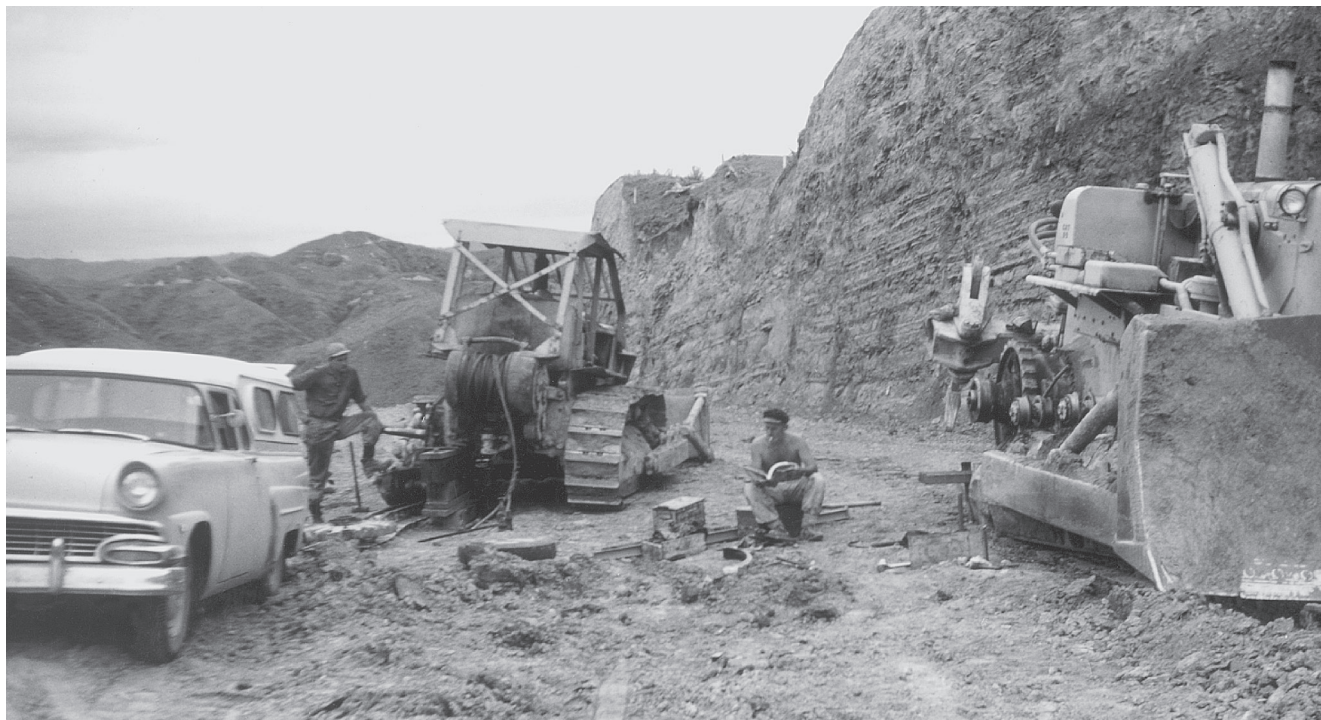
Two tractors in serious trouble! Both have final drive problems and the man in the middle must be perplexed as he is reading the service manual. The D7 on the left belonged to Frank McDonnell and it had stripped the teeth on the final drive gear. That is the pivot shaft visible near the man's knee. The D9 on the right was being assembled after it had broken the pivot shaft in the right-hand final drive. The track frame has yet to be fitted. Luckily it is dry weather.
