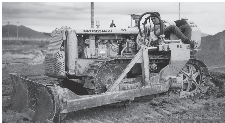
A Caterpillar D2 tractor on the scheme belonging to Des Ray. Small machines such as this one were used for cleaning up operations. The operator's name could not be recalled.
