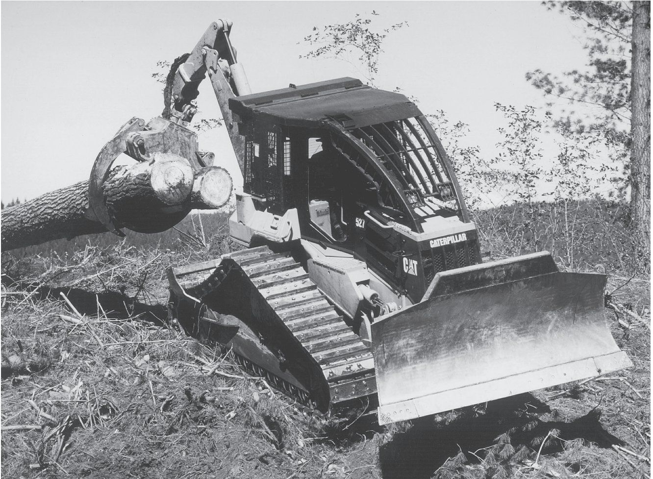
This is the latest type of tractor used for logging – a 527 Tracked Skidder belonging to Grace Brothers of Turangi. The machine is working in the Taupo Forest in 1999 and has a seven litre 3304 engine developing 150 hp and an operating weight of 21,500 kg including the blade and grapple. Compare this machine with the old RD8s shown in the earlier pages of this book which had a 20.4 litre engine developing 95 HP and an operating weight of 18,000 kg when equipped with a Hyster winch. It must be remembered however, that there is 60 years of technology between the two machines.
